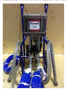
• TP2 and TP4SS Twin Piston Pneumatic Pumps
